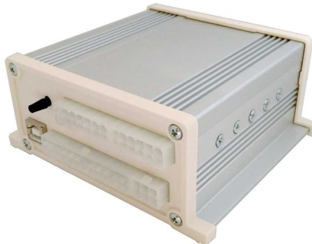
Fig. 5. The photo of the assembled SECU-3i EMS unit
