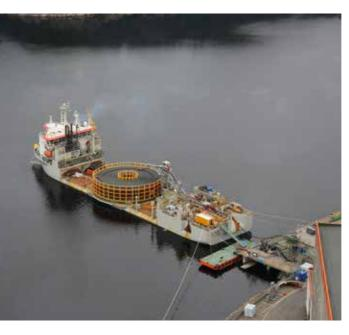
During the cable lay, the cable touchdown point was monitored by a separate vessel, fitted with a blue view and multibeam sonar and connected with a direct Wifi link to *Willem de Vlamingh*. As such the difficulties with TDM by ROV in shallow water were overcome and the responsible installation superintendent could review the real-time touch down information online
