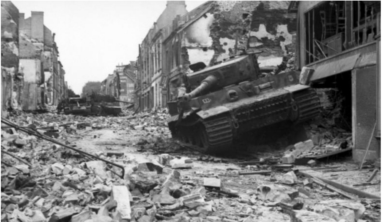
KNOCKED-OUT MONSTER This was Lt. Philipsen's Tiger which was likely destroyed by infantry fielding PIATs and Gammon bombs. Although the Tiger was heavily armed, its roof armour was weak, amounting to only 25mm thick — leaving it vulnerable to attack from above. Note the pair of a Tiger and Mk IV also knocked out further down the street.
