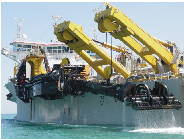
Figure 3. One of the 28 hopper dredgers of Jan De Nul Group. These vessels are used to dredge loose material and are able to excavate trenches up to 155 m deep.
