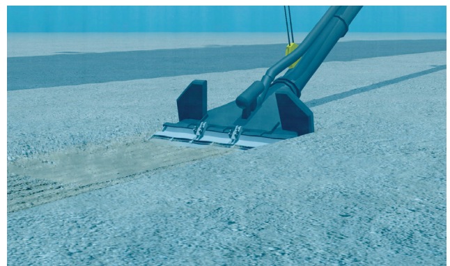
Figure 4. Simulation of a drag head used to dredge trenches for the installation of offshore pipelines.
