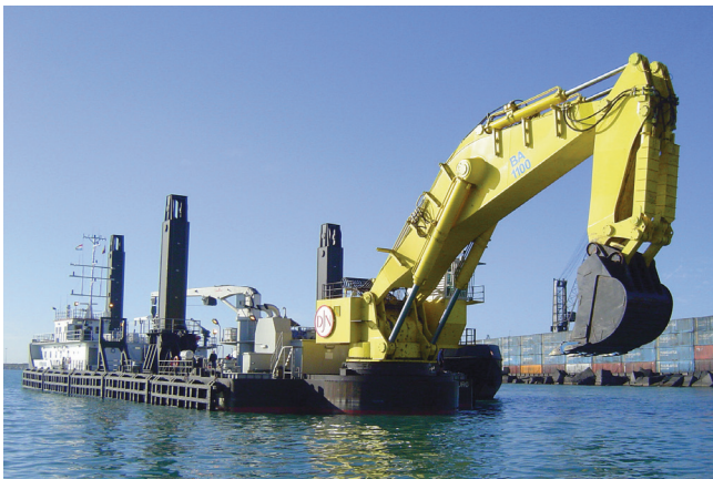
Figure 2. The backhoe dredger Vitruvius can be equipped with buckets with a grab capacity varying from 15 - 40 m 3 and is often used to dredge land approaches.
