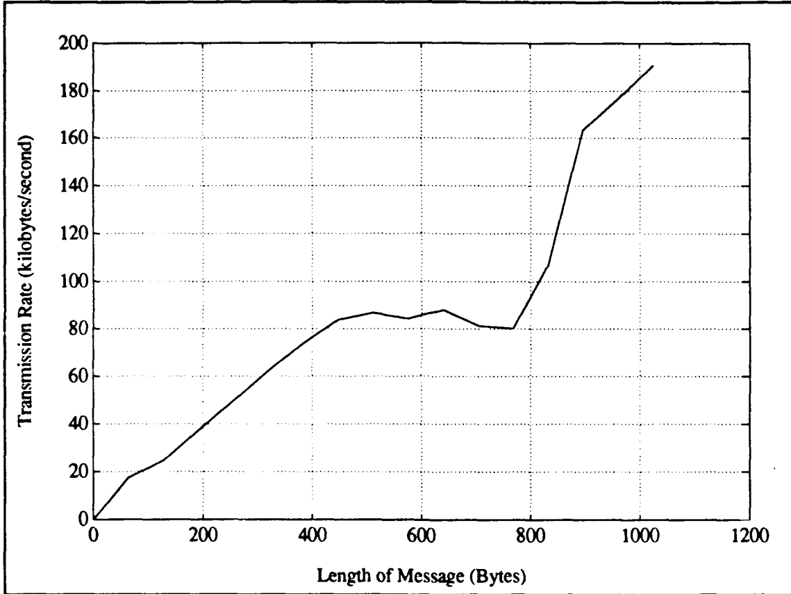
Figure E.3: Speed of Small Host-Node Messages (One Hundred Repetitions)
