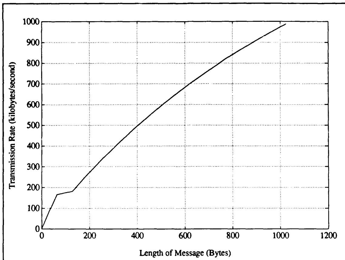
Figure E.4: Speed of Small Messages Between Nodes (One Hundred Repetitions)
