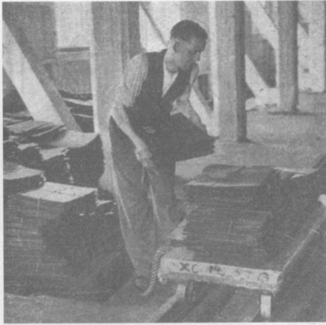
The raw material of steel helmets is seen above. Blanks from which they are stamped out are being piled on a truck which carries them to the press room.
