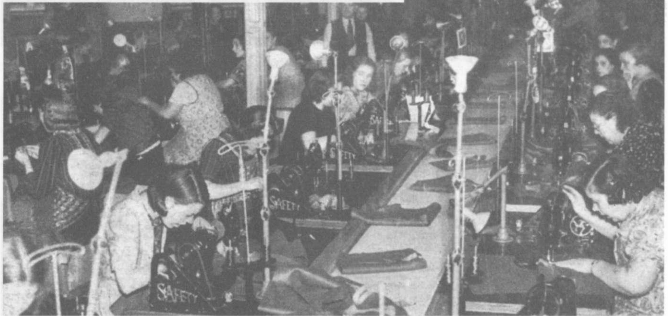
The first requirement for the soldier is his battledress, the new uniform that has the great advantage of doing away with puttees. Here women are at work in an Army clothing factory sewing uniforms with batteries of mechanically driven sewing machines. Centre left is a girl with a big pile of forage caps. The Royal Army Ordnance Corps is responsible for supplying every requirement of the Army, from guns and shells to clothes and boots, with the exception of food and transport, which fall within the province of the R.A.S.C. Photos, Central Press, Sport & General and Fox
