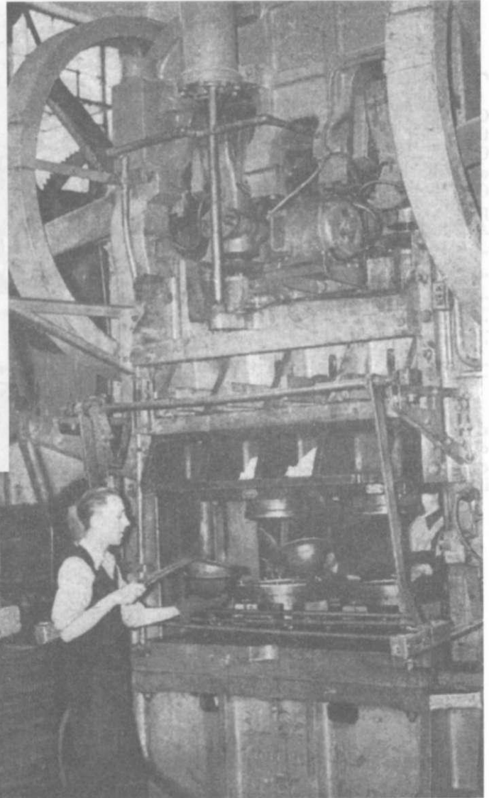
When the blank has been pressed into shape the next process is fitting the stainless steel rim. It is welded in position and then clinched home by the impressively powerful machine seen above.
