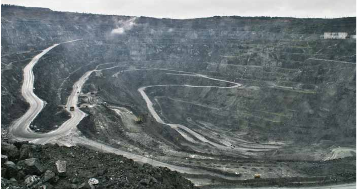
The Zhelezny open pit mine at Kovdor operates Atlas Copco and Russian drill rigs, Russian electric shovels and Belaz, Caterpillar and Komatsu haul trucks. The in-pit crushing station is on the upper right of the picture.
