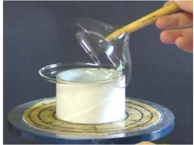
Plate 154 After a short time, the expansion of the glass caused by the heat from the flame has caused the conical top of the object to crack off horizontally all the way round. The unwanted upper dome portion (known as the moil) is set aside for recycling. This use of a hot flame jet is a modern method – in Roman times this very common task may have been achieved by applying a hot blade perhaps, or another of several similar techniques – no one knows for certain how this was done in antiquity
