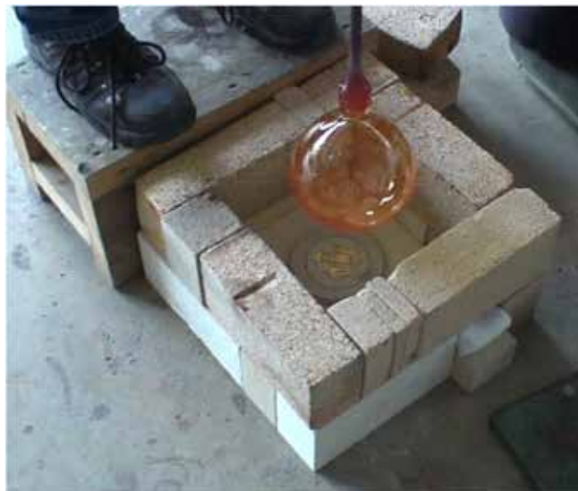
Plate 30 Fusing the gilded base-disc with the parison forming the vessel bowl
