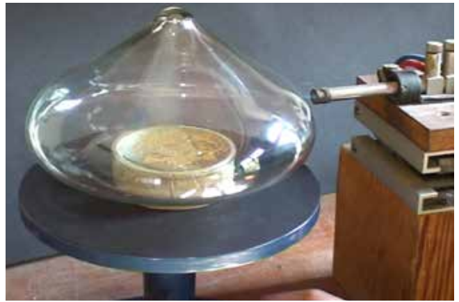
Plate 172 The edge of the complete bowl has a pencil flame played upon the area of the scored scratch, and is rotated on the wheel. After a few minutes, it will crack off due to the thermal shock
