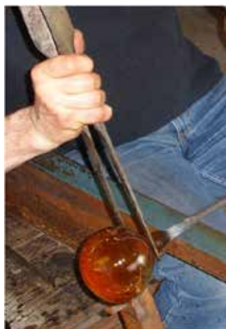
Plate 148 The glassblower gathers a small amount of hot colourless soda-lime glass from the main furnace onto the end of his blowing iron. The glass has been mixed to a Roman recipe, based upon analyses of original gold glass discs
