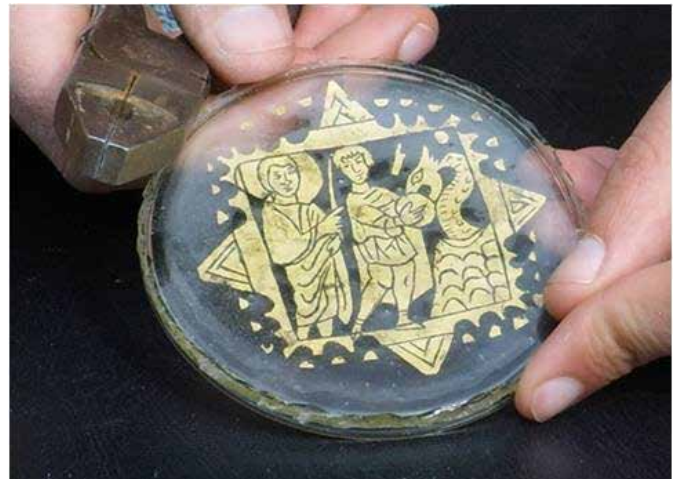
Plate 32a–b Grozing the vessel walls away to the line of the foot-ring (a) and the final product (b)
