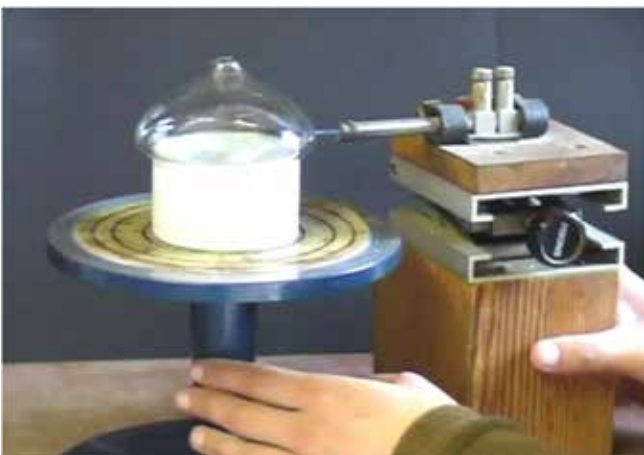
Plate 153 The foot-ring vessel is rotated on a wheel, whilst a pencil-point flame from a gas torch plays upon the scratch
