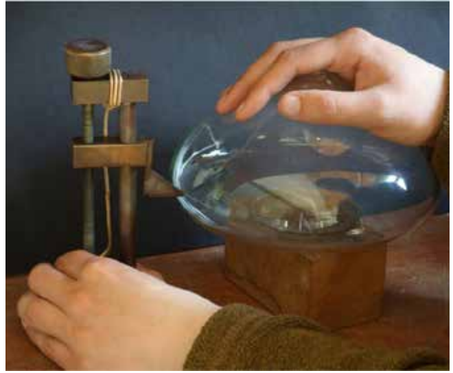
Plate 171 The edge of the bowl is scored with a diamond or sharp metal burr at the point where cracking off is desired
