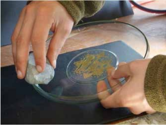
Plate 174 The finished bowl with its gold glass disc/foot-ring at the centre. The edge of the bowl may now be ground to remove its sharp edge, and the bowl will be complete
