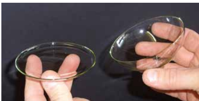
Plate 26 The base-disc and moil after the process of cracking off. The disc to the left is retained forming the pad base-disc, whilst the moil, seen to the right and forming the majority of the bubble, is recycled
