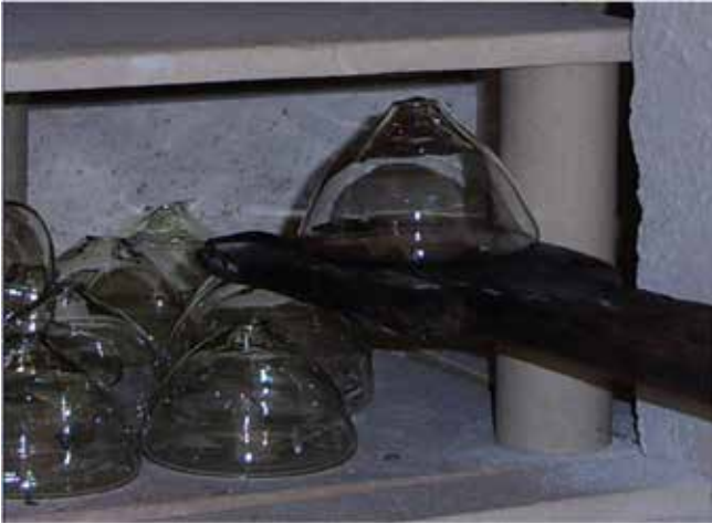
Plate 151 The finished blown 'proto-vessel' (which will become the base and foot-ring of a finished gold glass bowl) is cracked off from the blowing iron and placed into the annealing oven or 'lehr', which allows stresses in the glass resulting from uneven heating and cooling to dissipate by holding the glass at a steady temperature during the working day and slowly cooling it overnight
