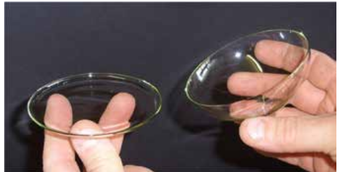
Plate 155 The two parts of the glass foot section – foot (left) and unwanted moil (right). The moil is destined to go back into the glass pot for remelting
