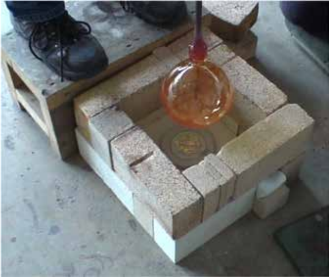
Plate 168 The glassblower has blown a large bubble of thin-walled glass, and after a reheating, lowers it onto the foot-ring so that the bowl glass covers and adheres to the surface
