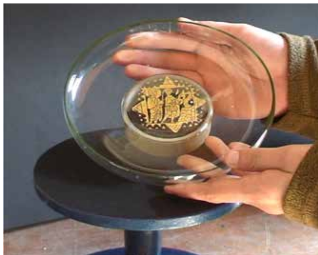
Plates 31a–b The vessel and its moil after the process of cracking off. The excess upper portion (the moil) is recycled (a), leaving a shallow bowl shaped vessel (b)
