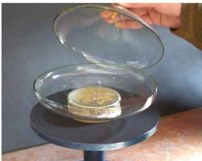
Plates 31a–b The vessel and its moil after the process of cracking off. The excess upper portion (the moil) is recycled (a), leaving a shallow bowl shaped vessel (b)
