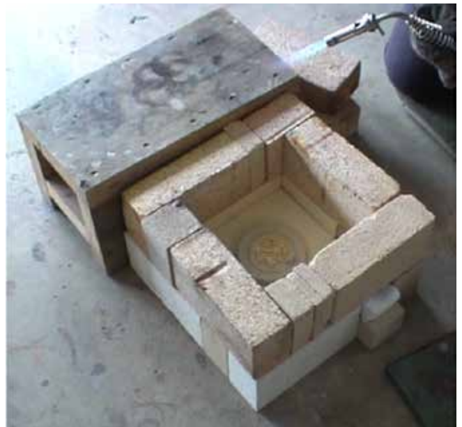
Plate 167 The assistant has placed the foot-ring into a small 'garage' of insulating bricks to prevent any draughts of cold air from allowing it to crack from thermal shock. As a double precaution, he is playing a gas torch onto the glass, so as to maintain its temperature at around 500°C
