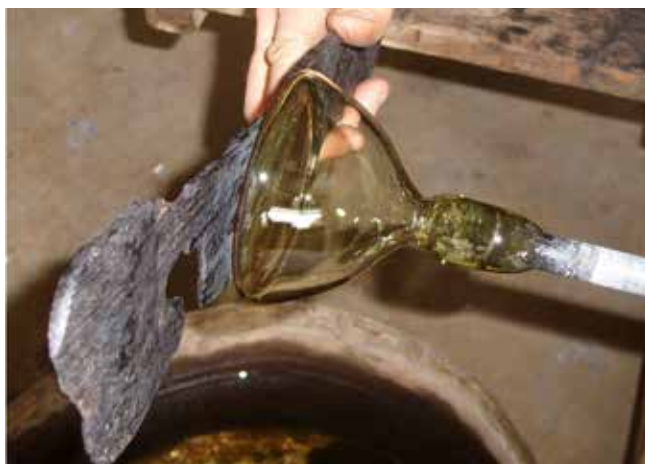
Plate 150 The base of the bubble has been pushed in and flattened using a flat piece of fruitwood, which is 'kinder' to the surface of the glass than metal tools
