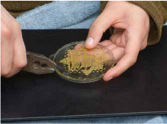
Plate 32a–b Grozing the vessel walls away to the line of the foot-ring (a) and the final product (b)
