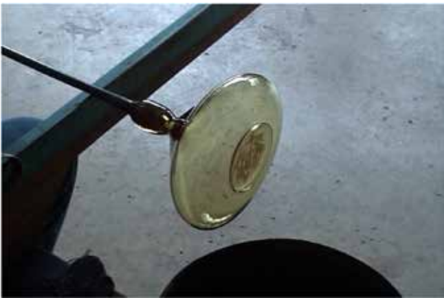
Plate 169 After reheating and shaping using gravity and centrifugal force, the glassblower now has a large bowl with the gold glass foot-ring/base bonded permanently at the bottom on his blowing iron. He will now crack this off at the neck, and place the domed 'vessel' in the lehr for annealing and overnight cooling
