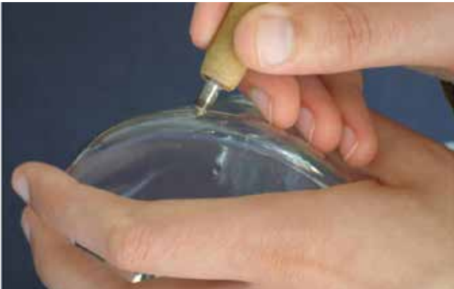
Plate 152 The now annealed (and cold) glass has a short (c. 5–10mm) scratch scored at its edge using a diamond or sharp metal burr, at a height where the foot and base will be cracked off. This will act as a 'crack-starter'
