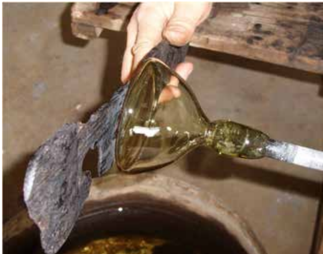
Plate 25a–b Shaping the base-disc parison
