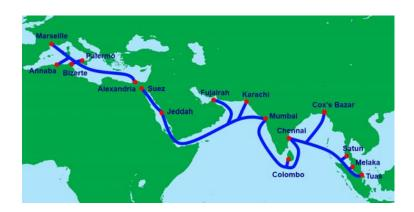
The SEA-ME-WE 4 Cable System, which was commissioned in 2005, is an ultra-high-capacity fiber optic submarine cable system linking South East Asia to Western Europe via the Middle East. The cable network, measuring approximately 20,000 kilometers and linking 16 landing stations, is owned by a consortium of 16 leading telecom carriers in 14 countries.
