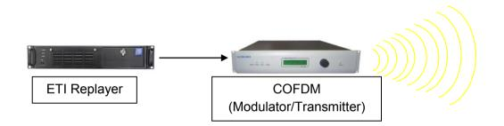
Some modulator/ transmitters that are designed for testing purposes incorporate an internal ETI Player. To play the ETI file you must upload it onto the lab modulator/ transmitter (e.g., via network or USB memory stick) and the lab modulator/transmitter directly plays the ETI file.
