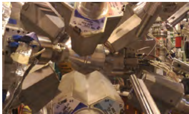
Figure 2. SPEDE spectrometer coupled to the MINIBALL gamma-ray spectrometer.
