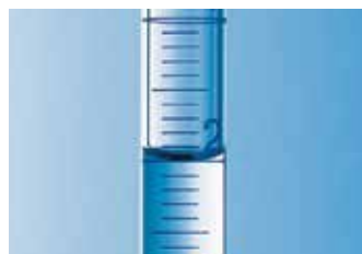
Concave meniscus in a graduated pipette.
