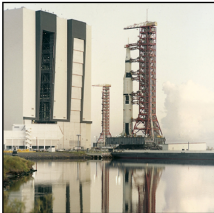
A Saturn V rocket rolls out of NASA's Vehicle Assembly Building on the crawler-transporter Aug. 1, 1967, for the Apollo 4 mission as seen from across the turn basin.
