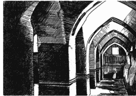
Fig.9. Massive column in the storage tank splits the space up into five contiguous spaces, Boshehr, Iran
