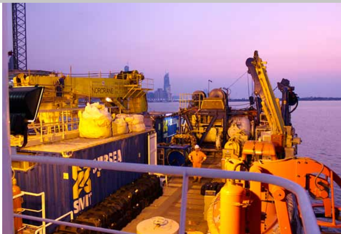
DP vessel 'Team Muscat' equipped with the six-man saturation dive system SMIT SAT3 for inspection work offshore Qatar.
