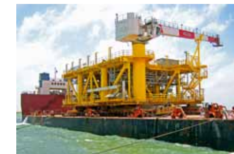
'Smit Anambas' loaded with the 2,000 tonnes Castor platform topsides.
