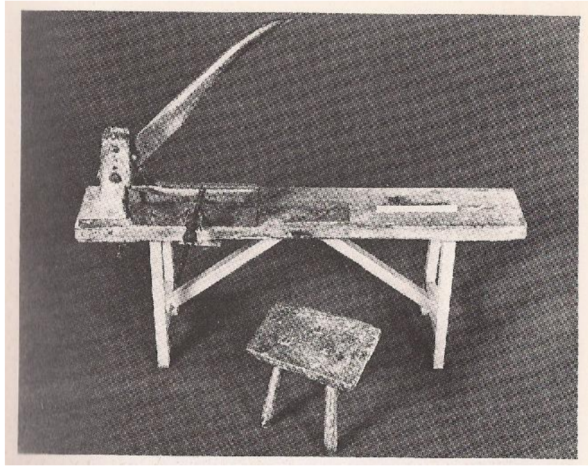
Figure 3.2: A photo of a gin-press. One of the few machines used in the production of pipes (source: Ayto, 1990, p. 22.).
