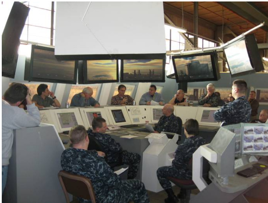
FIGURE 2 Zumwalt human factors engineers (HFE) needed only $5,000 in material to construct an accurate, highly detailed physical mock-up (from ship's drawings) of the bridge, ship's mission center, and Helo control station (HCS). These mock-ups were used multiple times by HW and SW teams as well as HSI.
