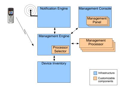
Figure 4 - Funambol Device Management Server architecture
