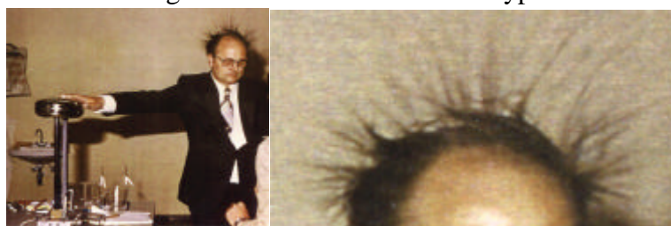
Figure 1. Hair disposition if a man (O. Scheuermann) is in contact with high-voltage electrostatic field produced by a Van de Graaff generator.
