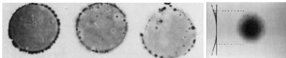
Figure 7. 3-D effect of coin images formed on photographic paper by means of CD. On the left, 3 coins were exposed to CD; the darker image corresponds to the coin closer to the condenser. On the right, a spherical object near a flat condenser generates an image darker in the middle showing 3-D effects.
