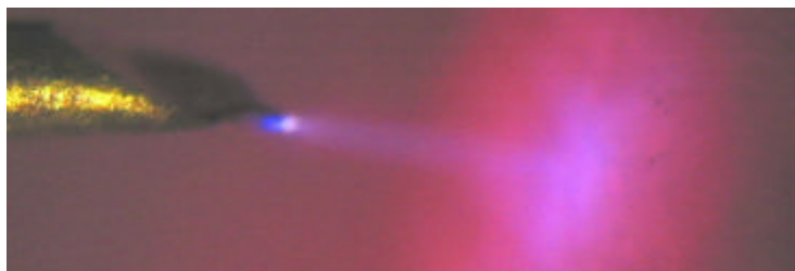
Figure 6. Positive CD in non-ionized air at a conductive point. The experiment involved a conductive point (left) in proximity to a plasma ball covered by a sheet of paper (right).
