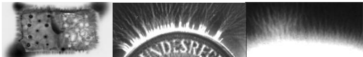
Figure 13. On the left, image of a 0.1 mm thick sheet of copper in which some convex hills (darker) and concave hollows (lighter) were previously made by means of a pointed stick. In the middle (positive CD) and on the right (negative CD), smear effects on coin images on photographic paper.
