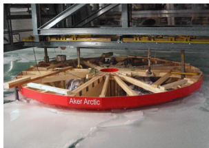
Arctic drilling platform Kulluk in model tests
