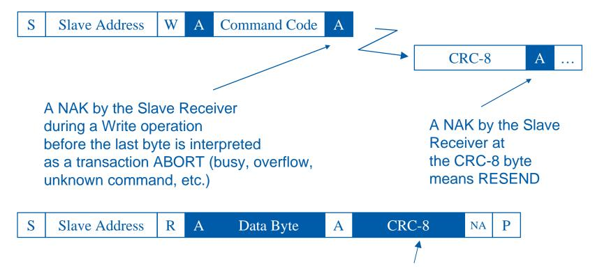
The Master Receiver detecting an error in the Packet Check Code, terminates the transaction and repeats the operation
