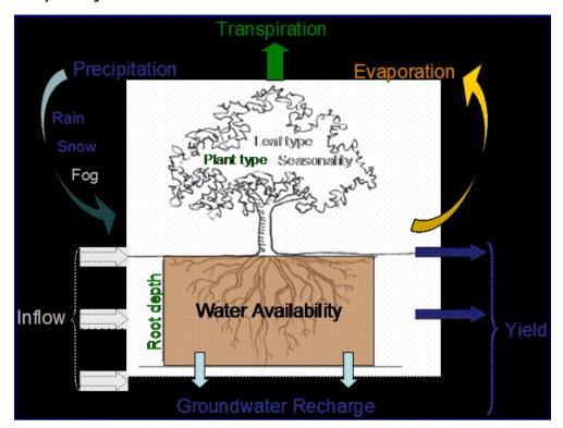
The conceptual diagram of the water balance model is used in the hydropower production model. The water cycle is simplified, including only the parametres shown in colour, and ignoring the parametres shown in grey (Figure 24).
