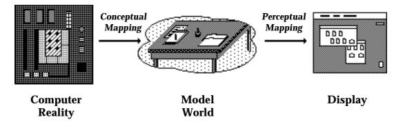
Figure 3. Two mappings exist between the reality of the computer and the display to which the user has access. The first is a conceptual mapping between events in the computer and those in some model world (for instance, that of a desktop). The second is a perceptual mapping between events in this model world and their perceptible manifestations, be they visual or auditory.
