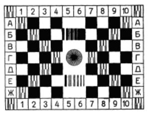
First test chart for TV paths testing according to the 625 line standard
