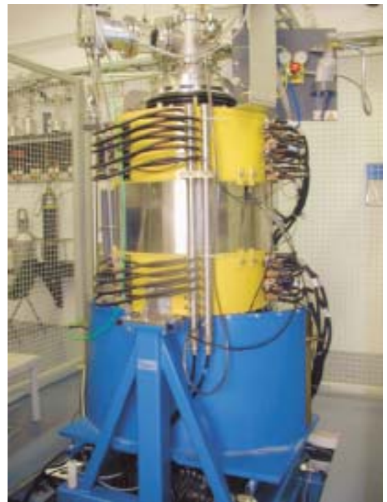
Fig. 2. The upgraded 6.4 GHz ECR ion source.
