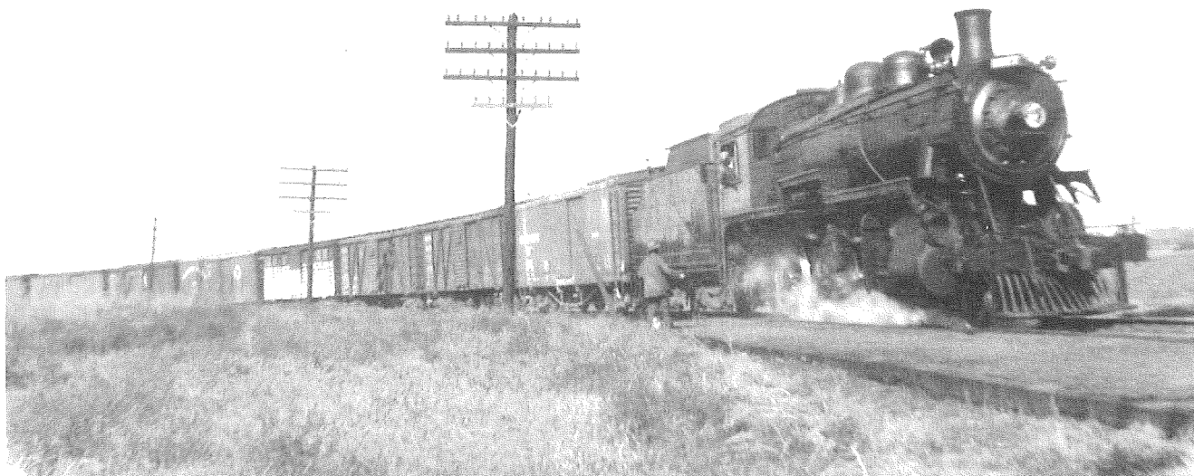
CP 4-6-0 No. 1027 approaches Ottawa West Station after coming off the Prince of Wales Bridge from Hull in 1950. Note the older types of boxcars all made of wood including some with outside bracing. Bruce Chapman collection.
