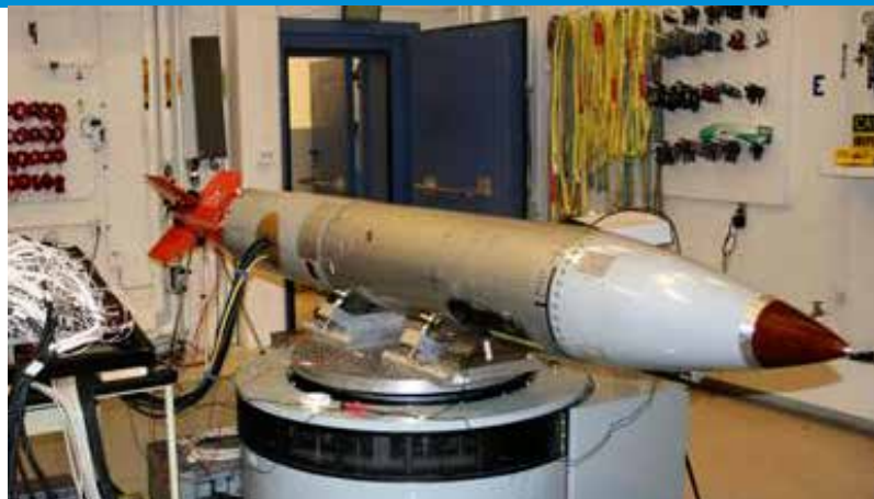
In February 2014, NNSA announced that Los Alamos and Sandia national laboratories successfully completed the first full-system mechanical environment test of the B61-12 as part of the NNSA's ongoing effort to refurbish the B61 nuclear bomb.
