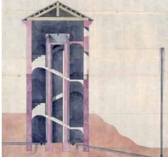
Fig.2 - On the left, a modern reconstruction drawing of the Fountains of the Ducal Garden of Colorno; on the right, a drawing of the hydraulic gimmick inside the tower probably used to pump in the water (conserved in Fondazione Cariparma)
