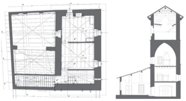
Fig.4 The structural survey of the first floor, with the indication of the beam warpings transversal section of the tower and of the near mill (Torchio)
