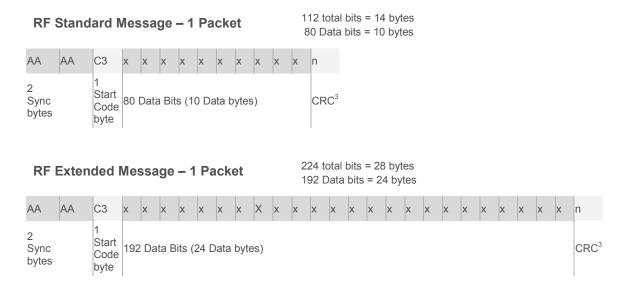
It takes 2.708 milliseconds to send a 104-bit Standard message, and 5.625 milliseconds to send a 216-bit Extended message. Zero crossings on the powerline occur every 8.333 milliseconds, so a Standard or Extended RF message can be sent during one powerline half-cycle. The waiting times after sending powerline messages, as shown in the section Powerline Packets, are to allow sufficient time for INSTEON RF devices, if present, to retransmit a message.
