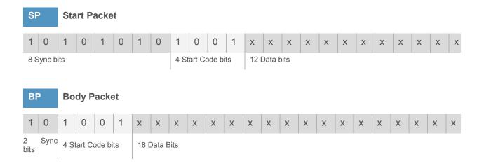
Powerline packets begin with a series of *Sync Bits*. There are eight Sync Bits in a Start Packet and there are two Sync Bits in a Body Packet. The alternating pattern of ones and zeros allows the receiver to detect the presence of a signal.
