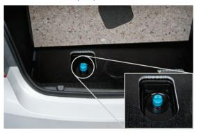
Your vehicle is equipped with a 4.8-gallon DEF tank that is accessible by lifting the load floor in the trunk. DEF is used with diesel engines to reduce the amount of regulated emissions produced. The fluid level in the DEF tank must be maintained for the vehicle to run correctly.
