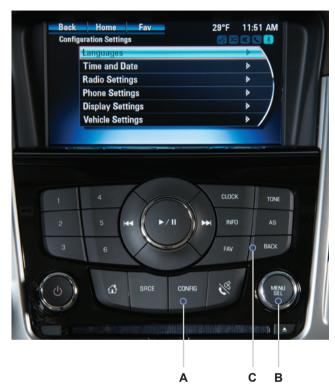
Some vehicle features can be customized by using the audio controls and menus. Personalization menus may include Climate and Air Quality, Comfort and Convenience. Collision/Detection Systems, Lighting, Power Door Locks. Remote Lock/ Unlock/Start, and Factory Settings.
