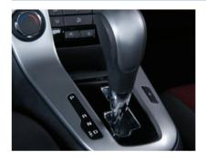
**Note:** The transmission has a fuel-saving Neutral shift feature. It shifts into Neutral when the vehicle comes to a stop and the brake pedal is applied. It shifts back to Drive when the brake pedal is released. When stopped on a hill, the vehicle may roll very slightly before shifting into Drive.
