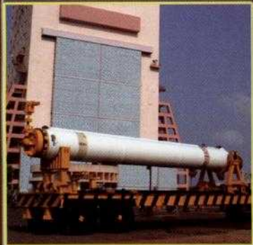
Strap-on stacking at VAB
