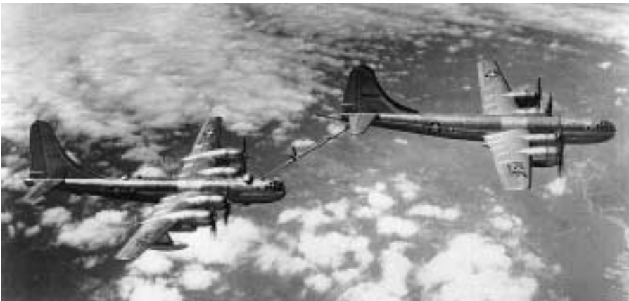
The photo depicts a B-50 bomber refueled by a KB-29 tanker on 24 July 1950. SAC concentrated on developing an intercontinental strike force. Aerial refueling also extended the range of RB-50 Ferret aircraft.
