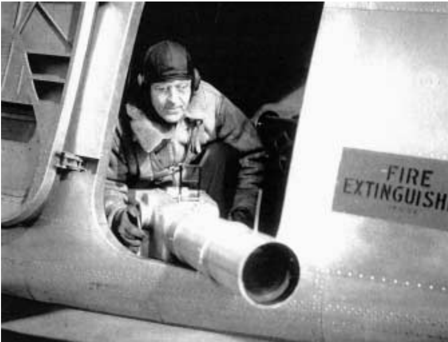
Col George W. Goddard operates a K-15A camera. He pioneered the development of the 48-, 60-, and 100-inch focal-length cameras in the late 1940s.
