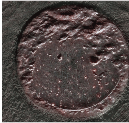
Figure 6-9. A dust free, cleaned and smoothed surface provides a better target for instrument measurements than an “as-is” surface.
