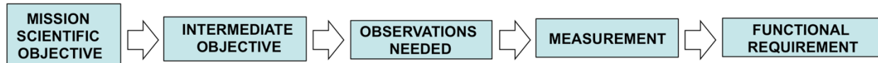
Figure 3-7. Traceability Matrix “road map.” The minimum suite of measurements necessary to address the mission objectives must flow from those objectives in the manner shown.
