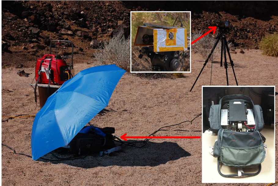
FIG. 4. The TextureCam single-camera field instrument consists of a tripod-mounted camera with sunshade (upper inset) and a backpack-mounted DPU and control computer (lower inset).
