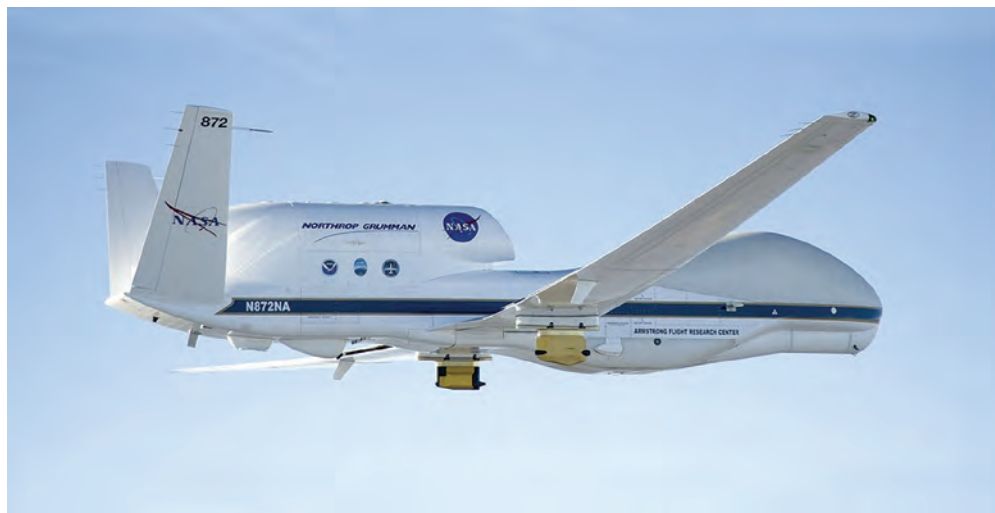
FIGURE 26 NASA Global Hawk shown with the CAST AIIITS and ATTREX Hawkeye instruments on the wing pylons.
