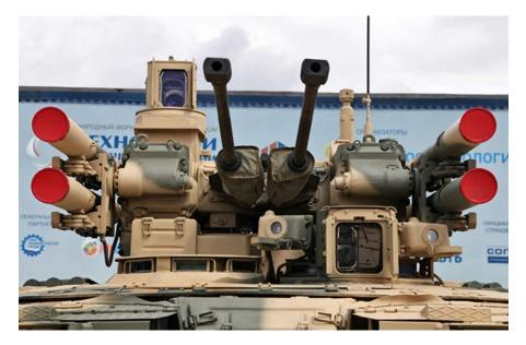
Figure 3. The commander's panoramic sight (located on the roof) gives the BMPT hunter-killer capabilities by continuously scanning targets for the gunner. (*Photo copyright Vitaly Kuzmin, http://vitalykuzmin.net. Licensed under a Creative Commons Attribution-ShareAlike 3.0 Unported License*)
