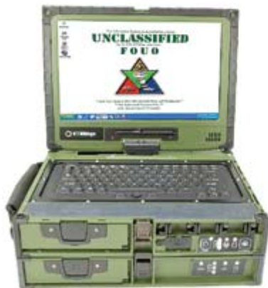
Maintenance Support Device- Version 3 (Type 1) with docking station
