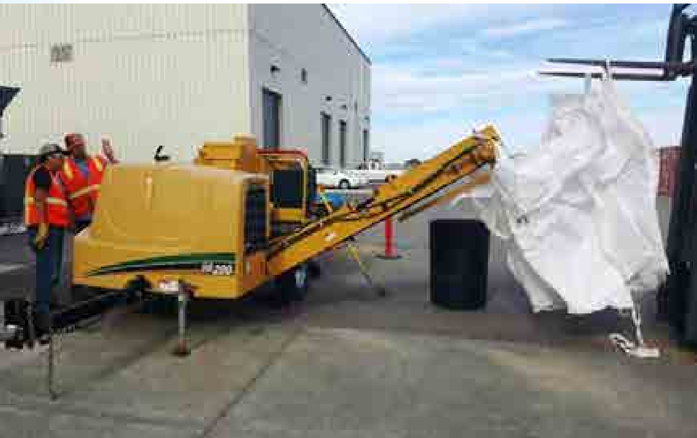
Juniper sample being ground up using Vermeer HG 200 horizontal hammermill grinder by INL's Biomass Feedstock Characterization team.
