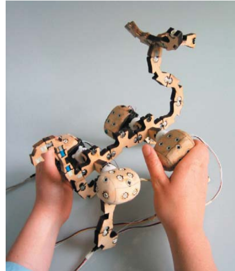
Figure 146 – Topobo: programming a horse to walk
