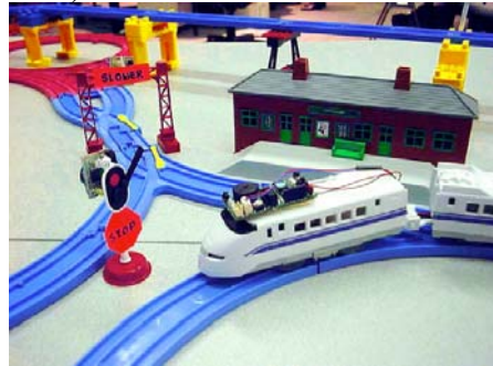
Figure 133 – Train set augmented with a Cricket programmable brick to heed infrared beacon signs
