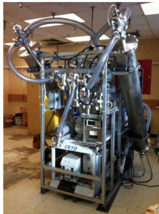
Deradnator can deliver 0.85 \text{ m}^3/\text{min} of low Rn air
