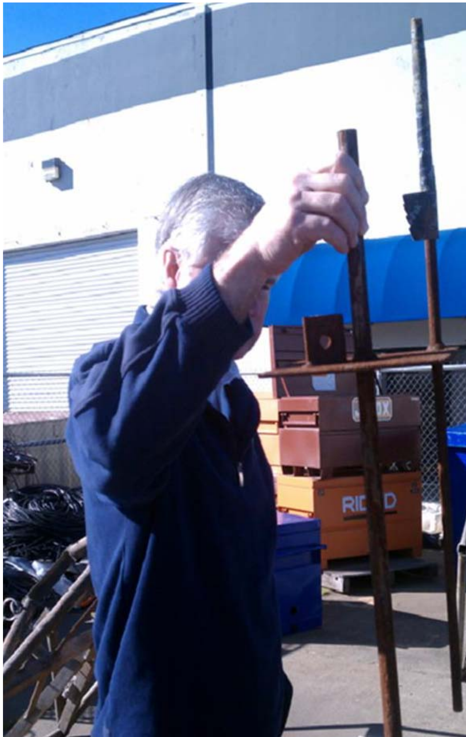
Figure 2-7 Representative Photograph of a “Pound-In” Mount
