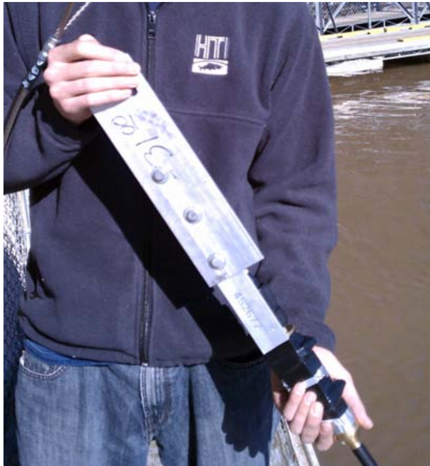
Figure 2-8 Representative Photograph of a “Dock” Mount
