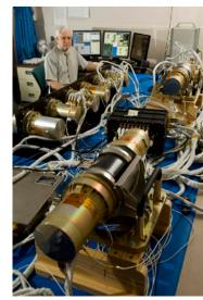
GLAST Burst Monitor Principal Investigator Charles "Chip" Meegan, an astrophysicist at NASA's Marshall Space Flight Center in Huntsville, Ala., tests the GLAST Burst Monitor. Credit: NASA/MSFC/ D. Higginbotham
