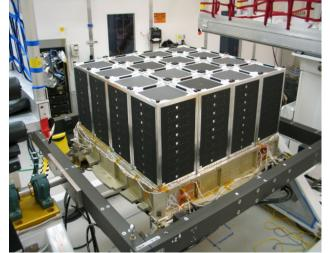
The LAT has 16 towers of particle detectors, seen here before the installation of the Anticoincidence Detector. Each tower contains a Tracker module and a Calorimeter module. The Data Acquisition System is located underneath the towers.
