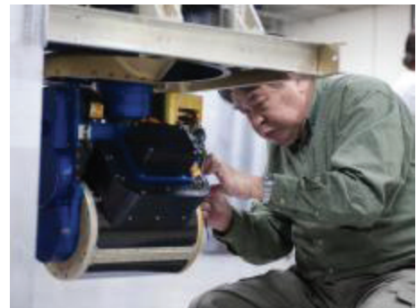
NASA Goddard engineer Zhaonan Zhang adjusts the Conical Scanning Millimeter-wave Imaging Radiometer, or CoSMIR, scan head prior to installation in NASA’s DC-8 flying science laboratory. The instrument is being used in the GCPEX airborne study of snowfall in Canada and the northeastern United States. Credit: NASA / Tom Tschida
