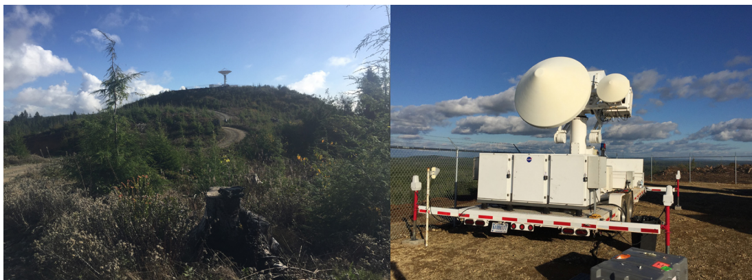
Figure 2.21: NPOL (left) and D3R (right) radars shown deployed along the coast Pacific Ocean near Moclips, Washington. Both radars operated nominally and provided high-quality, multi-frequency (S-, Ka-, and Ku-band) observations of rain, mixed-phase and ice (snow) precipitation.
