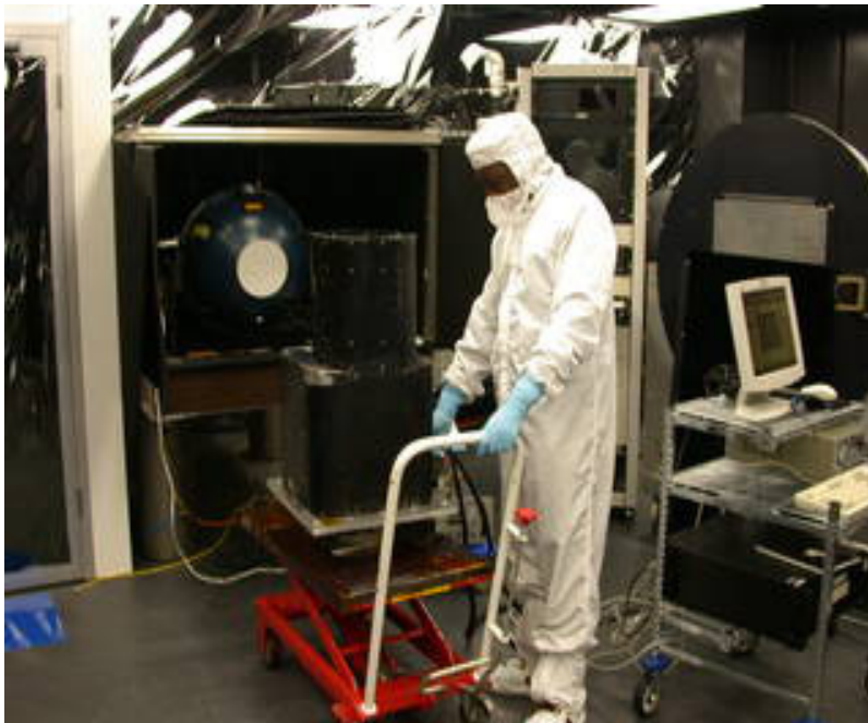
Gatebe preparing the CAR instrument (on the cart) for calibration with an integrating sphere in Goddard's Calibration Facility in Building 33.
