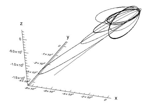
Trajectory of the Cassini vehicle in the J2000 frame, for June 20, 2004 to Dec 1, 2005
