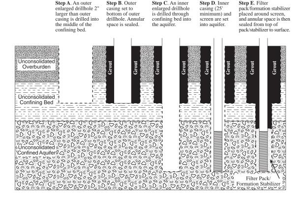
Figure 11a. Rotary method for flowing well construction where both confining bed and aquifer are unconsolidated-double casing construction.
