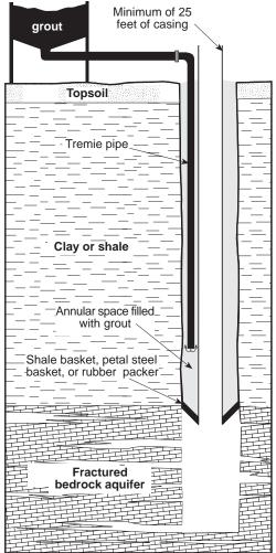
Figure 12. Recommended grouting procedures for wells penetrating fractured or cavernous formations.
