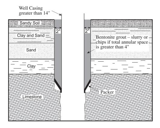
Figure 4b. Example of recommended rotary-drilled well construction for wells developed in consolidated formations—total annular space 4 inches or more.
