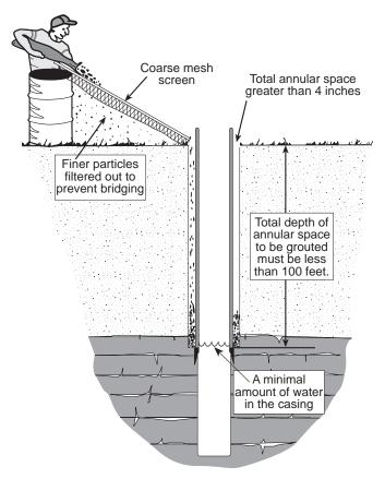
Figure 7. Grouting the annular space of wells with coarse grade bentonite products using the pouring method. (Modified from Wisconsin Department of Natural Resources, 1993)
