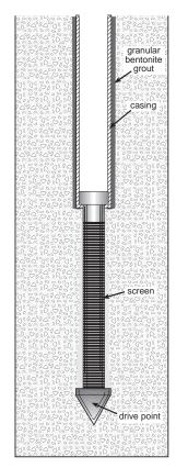
Figure 6. Example of recommended driven well construction.
