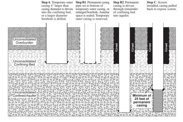
Figure 11a. Cable tool method for flowing well construction-confined unconsolidated aquifer with an unconsolidated confining bed.
