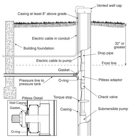
Figure 14. Example of pitless adapter installation.
