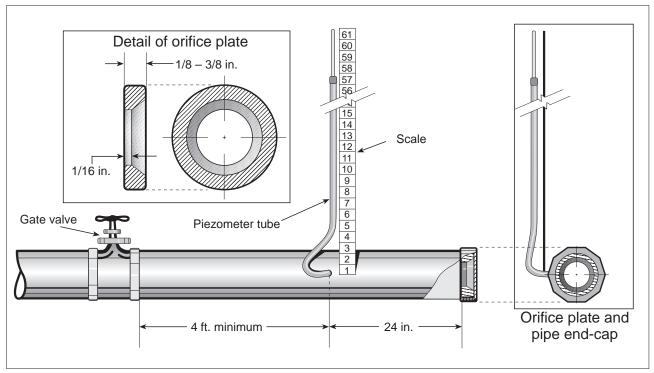
Figure 2. Detail of orifice weir construction.
