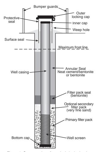
Figure 1. Cross-section of a typical single-riser/limited interval monitoring well.
