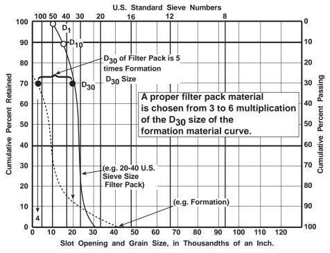
Figure 3. Selection of screen slot size based on the filter pack grain size. (Source: Design and Installation of Ground Water Monitoring Wells by D.M. Nielsen and R. Schalla, Practical Handbook of Ground Water Monitoring, edited by David M. Nielsen, Copyright 1991 by Lewis Publishers, an imprint of CRC Press. Boca Raton, Florida, With permission.)
