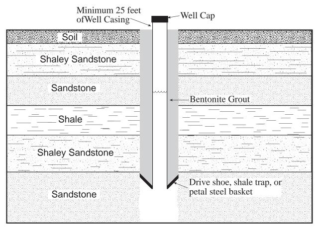
Figure 9b. Recommended well construction for wells penetrating multiple consolidated aquifers.
