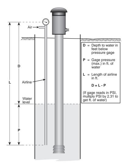
Figure 1. Example of airline setup and operation.
