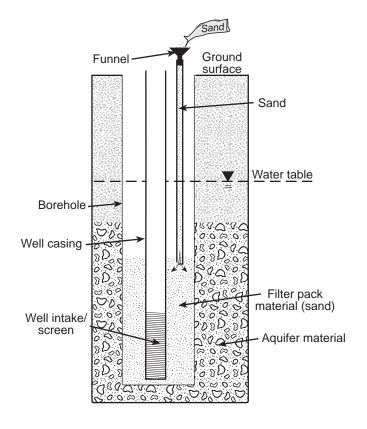
Figure 4. Tremie pipe emplacement of annular seal material. (Source: Design and Installation of Ground Water Monitoring Wells by D.M. Nielsen and R. Schalla, Practical Handbook of Ground Water Monitoring, edited by David M. Nielsen, Copyright 1991 by Lewis Publishers Division, an imprint of CRC Press, Boca Raton, Florida. With permission.)
