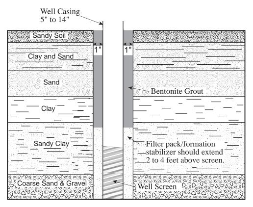
Figure 4a. Example of recommended rotary-drilled well construction for wells developed in unconsolidated formations—total annular space 2 inches or more.
