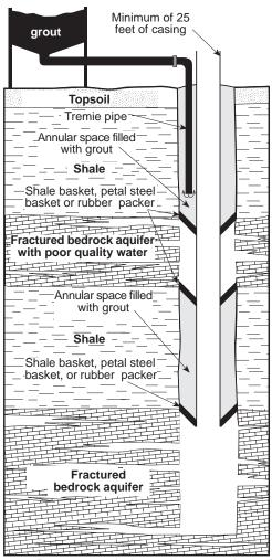
Figure 13. Recommended grouting procedures for wells penetrating fractured or cavernous formations where an upper fractured or cavernous zone has been sealed off.
