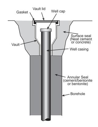
Figure 5. Typical flush-to-ground monitoring well completion. (Source: Design and Installation of Ground Water Monitoring Wells by D.M. Nielsen and R. Schalla, Practical Handbook of Ground Water Monitoring, edited by David M. Nielsen, Copyright 1991 by Lewis Publishers Division, an imprint of CRC Press, Boca Raton, Florida. With permission.)
