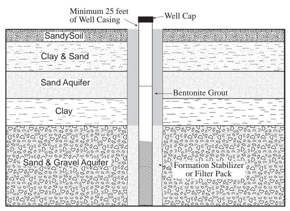
Figure 9a. Recommended well construction for wells penetrating multiple unconsolidated aquifers.
