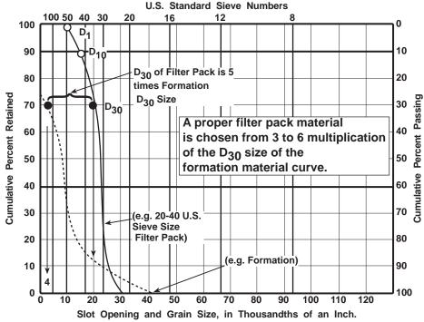
Figure 2. Artificial filter pack design criteria (Source: Design and Installation of Ground Water Monitoring Wells by D.M. Nielsen and R. Schalla, Practical Handbook of Ground Water Monitoring, edited by David M. Nielsen, Copyright 1991 by Lewis Publishers, an imprint of CRC Press, Boca Raton, Florida. With permission.)
