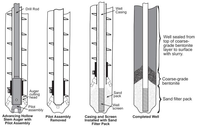
Figure 5. Example of well construction using hollow stem augers. (Modified from Hackett, 1987 and 1988)
