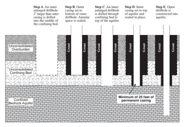
Figure 10a. Rotary method for flowing well construction-confined bedrock aquifer with an unconsolidated confining bed.
