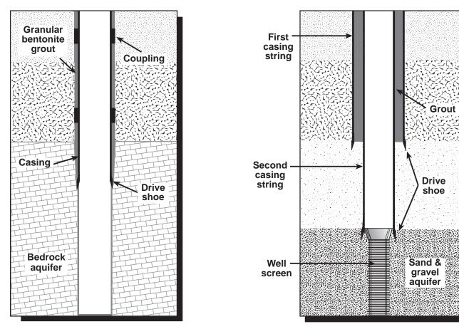
Figure 3. Examples of recommended well construction using cable tool drilling methods.
