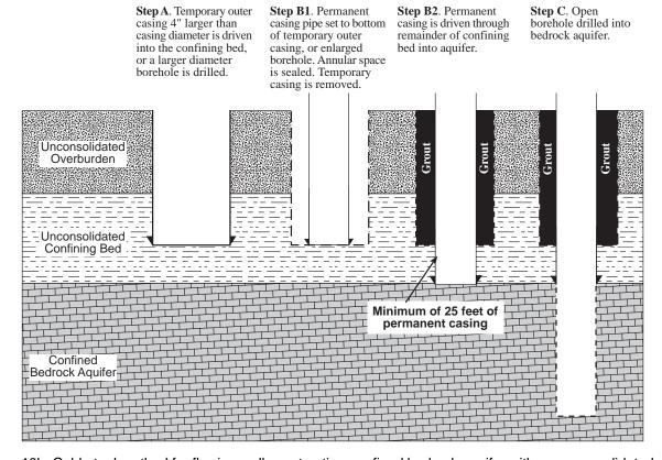
Figure 10b. Cable tool method for flowing well construction-confined bedrock aquifer with an unconsolidated confining bed.
