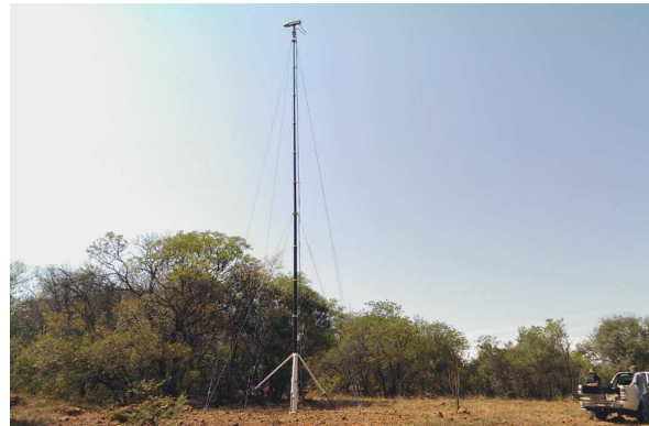
Fig. 6 Philip's rig for measuring RFI at the proposed VGOS site.
