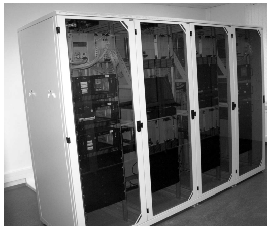
Fig. 1 View of the six-station ARC correlator, showing four racks containing (left to right) signal distribution and synchronization system (SDSS) and three Mark 5B playback units, two correlator crates and a KVM, three correlator crates, and one more cabinet with an SDSS and three Mark 5B playback units.
