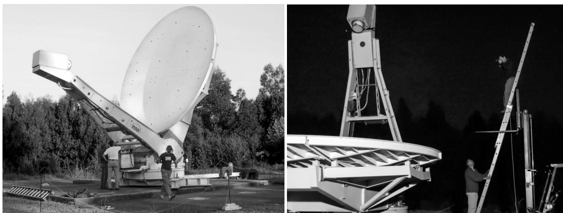
Fig. 3 (Left) The VLBI telescope primary mirror covered with reflecting targets for photogrammetry measurements. (Right) Pictures taken at different angles with the telescope pointing at 110 degrees of elevation. Credits: Rolando Dünner/AIUC.
