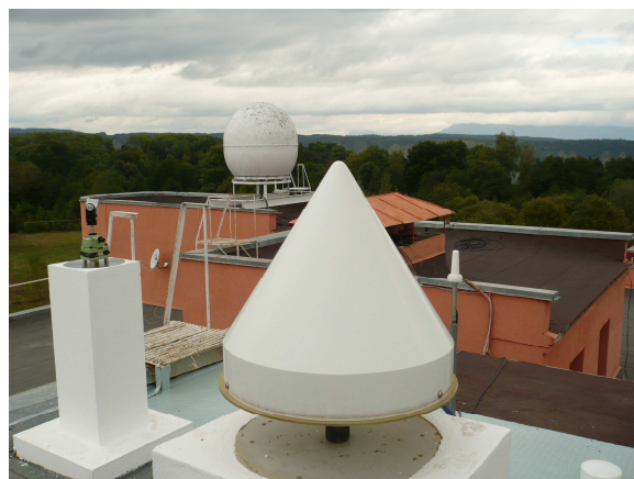
Fig. 2 Javad GPS/GLONASS/Galileo receiver at the Zelenchukskaya observatory.
