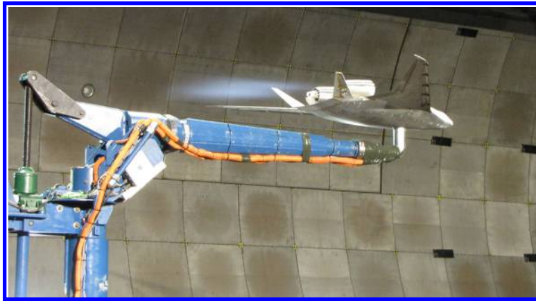
Figure 9: HWB model (turbine powered simulator configuration) operating statically in the NFAC 40- by 80-foot test section.
