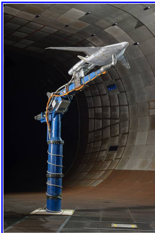
Figure 8: HWB model (ejector configuration) installed in the NFAC 40- by 80-foot test section.
