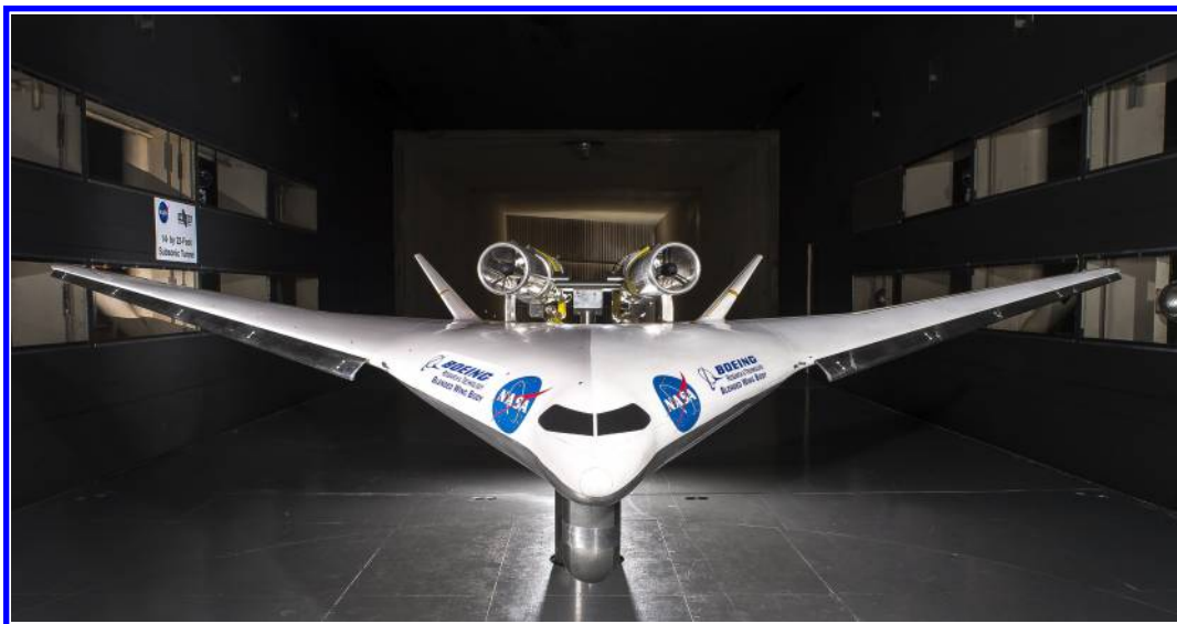
Figure 13: HWB model (ejector configuration) installed in the NASA LaRC 14- by 22-foot Subsonic Tunnel.
