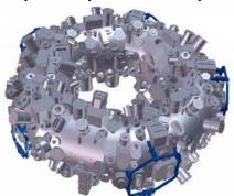
Figure 2: PPPL/ORNL are designing and building five normal-conducting trim coils, which will allow individual adjustment of the divertor heat patterns in the five modules of W7-X. Shown is a CAD drawing of the W7-X outer vacuum vessel, with attached trim coils (in blue).
