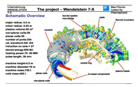
Figure 1: A schematic of the superconducting W7-X stellarator, presently under construction in Greifswald, Germany, and a table of design parameters.
