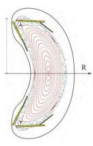
Figure 3: Divertor scraper elements will protect the throat (narrowest part) of the divertor against heat transients during evolution of the plasma beta. The magnetic configuration near the island divertor plates is shown on the right.
