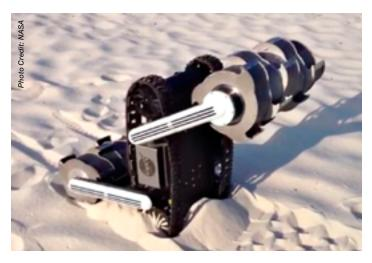
With a pair of drums positioned on arms, RASSOR can take on a number of different shapes to accomplish its work.
